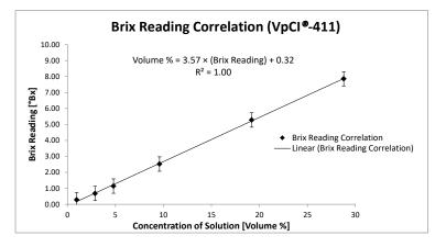
Please note the solutions used above were created using deionized water. Slight differences in water chemistry (dissolved solids, hardness, etc.) may lead to differences in readings. Please use these numbers as reference only. Contact Cortec<sup>®</sup> Technical Service with any questions
